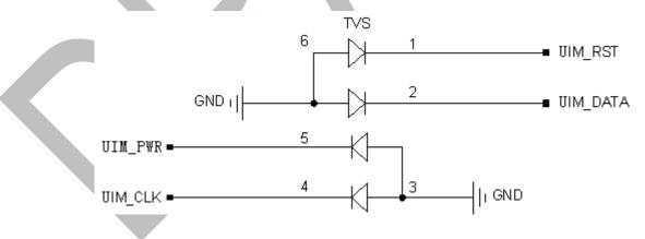
Figure 3-11 ESD protection circuit on the UIM card
